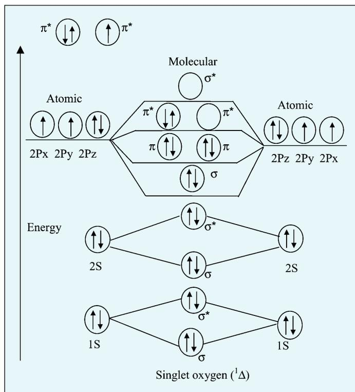
**Figure 2—Molecular orbitals of singlet oxygen and superoxide anion**
