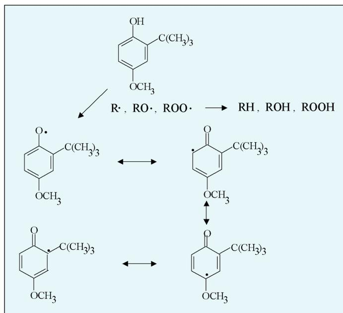
**Figure 6—Resonance stabilization of phenolic antioxidant radicals. Antioxidant radicals are stabilized through resonance structures.**
